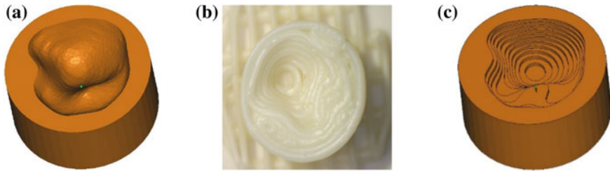
Fig. 3 a STL model of guide, b image of fabricated guide (FDM) SH = 0.3 mm, c sliced CAD model with slice height = 0.3 mm
