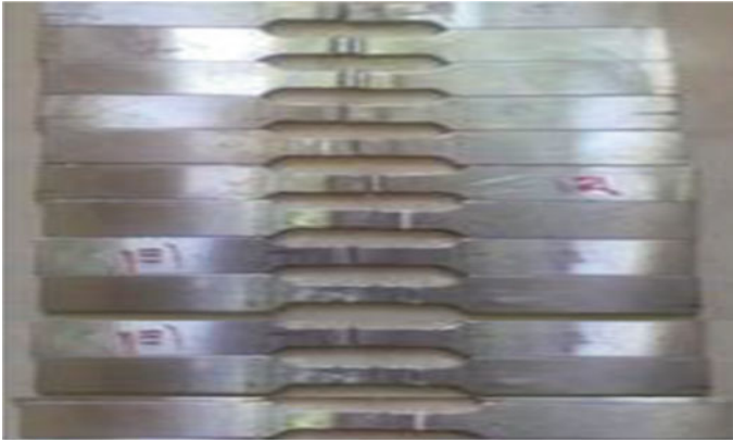
Fig. 4 Location of weld direction in tensile test specimen
