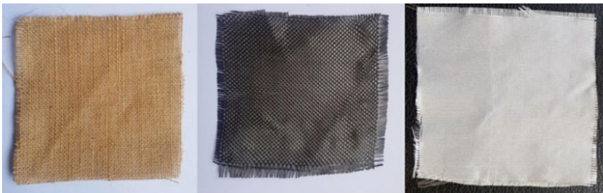
Fig. 1 Flax, carbon, and E-glass fiber mats
