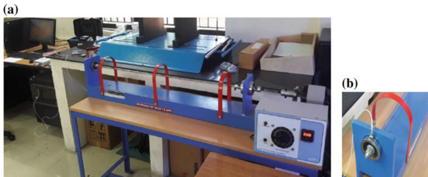
Fig. 1 a Experimental setup for the vibrational analysis of the rolling contact bearings. b Left-hand side faulty bearing with the accelerometer placed at its head attachment
